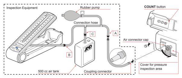
1. Hold the **COUNT** button on the rear of the blood pressure monitor, and turn the **POWER** switch on.
