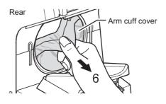
Insert the new arm cuff cover and push the vinyl ring into the groove (on the inner side of the frame) to attach.
