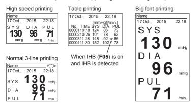
Note: In the table printing mode, paper is not cut automatically. To cut paper, hold the ▲ button for 2 seconds while the monitor is in the standby mode.
