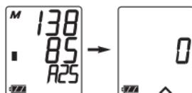
6. Press the exhaust valve until the ▲ mark is displayed. Squeeze bulb repeatedly until the ▲ mark disappears.
